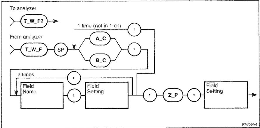
*Fig. 6.18 Syntax for the T\_W\_F? query message and analyzer response*
