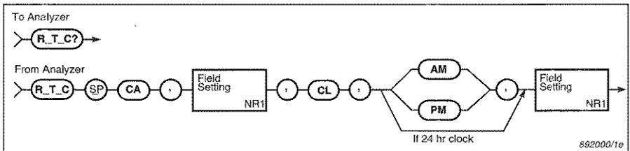
Fig.6.20 Syntax for the **R\_T\_C?** query message and analyzer response
