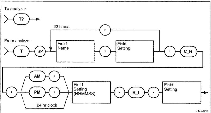
Fig. 6.28 Syntax for the T? query message and analyzer response
