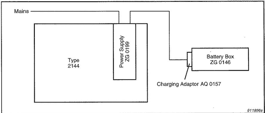
*Fig.2.2 Arrangement for simultaneous powering and recharging*
