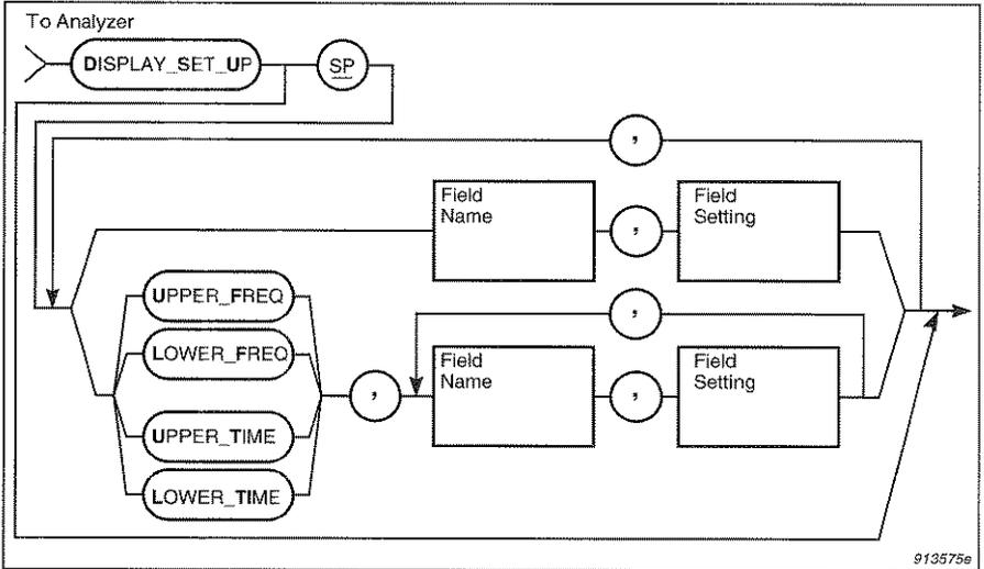
Fig. 6.13 Syntax for the **D\_S\_U** command message
