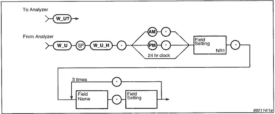
*Fig. 6.22 Syntax for the W\_U? query message and analyzer response*
