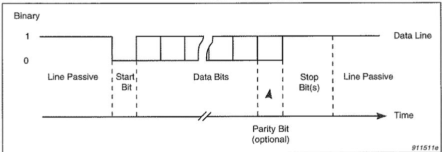
*Fig.3.2 Asynchronous transmission of 1 byte of data*
