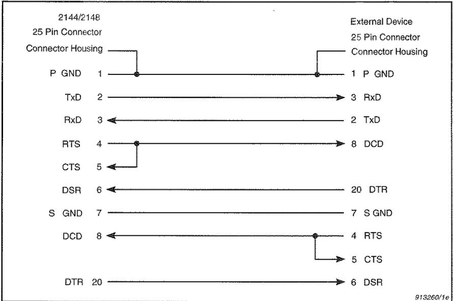
*Fig. 3.3 Null-modem cable with 25-pin connectors at both ends (Brüel&Kjær order numbers WL0946 and WL0947)*
