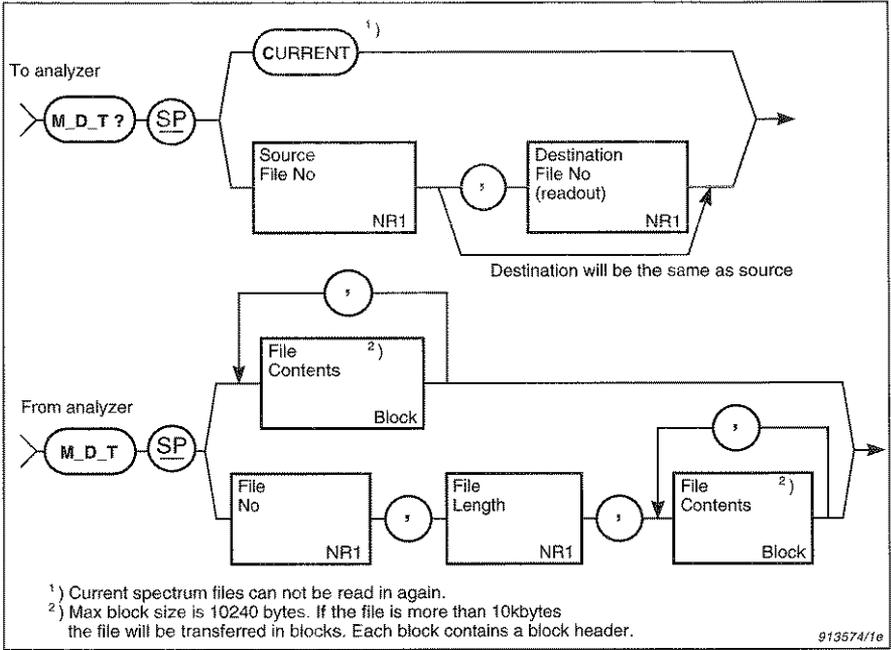
*Fig.8.5 Syntax for the **M\_D\_T?** query message and analyzer response*
