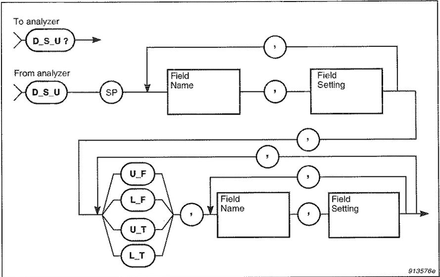
*Fig.6.14 Syntax for the **D\_S\_U?** query message and analyzer response*
