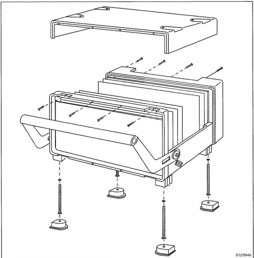
*Fig.2.5 Dismantling the analyzer*
