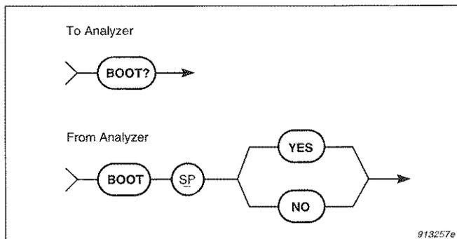
*Fig. 5.4 Syntax for the **BOOT?** query message and analyzer response*
