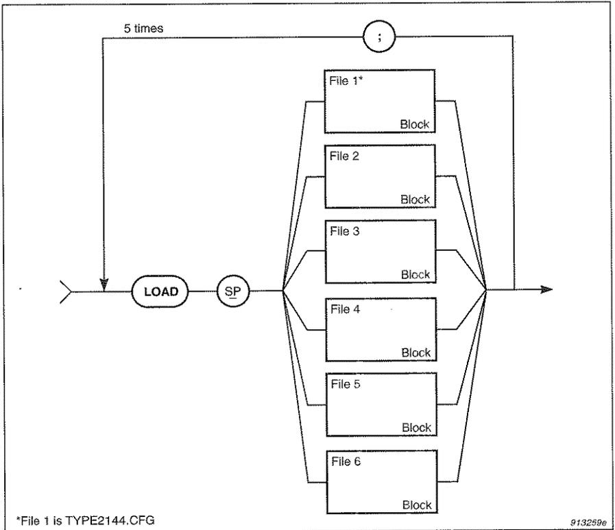
*Fig.5.6 Syntax for the **LOAD** command message*
