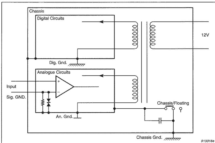
*Fig. 2.3 Simplified circuit diagram showing the grounding principle of Type 2148 (one input channel shown)*
