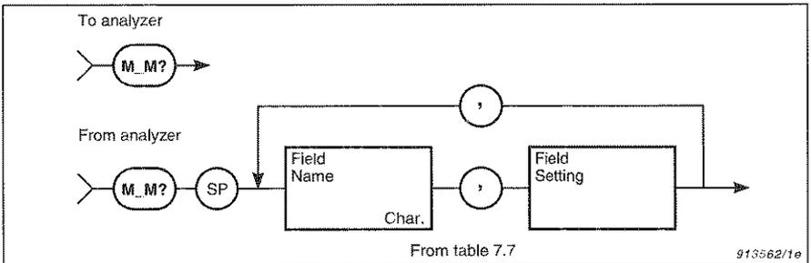
Fig. 7.12 Syntax for the **M\_M** query message and analyzer response
