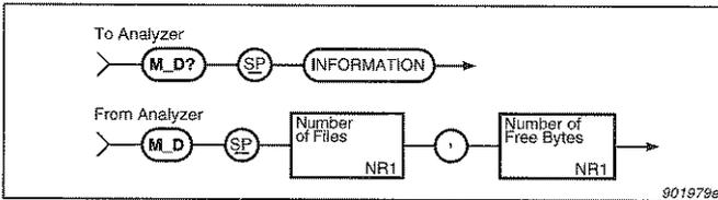
Fig. 6.32 Syntax for the **M\_D?** Information query message and analyzer response
