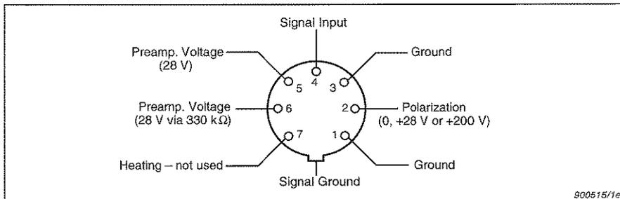
Fig. 3.5 Pin designation for 7-pin preamplifier connector (outside view)
