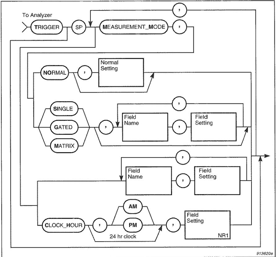
Fig. 6.26 Syntax for the **T** command message. For Normal Setting see Fig. 6.31
