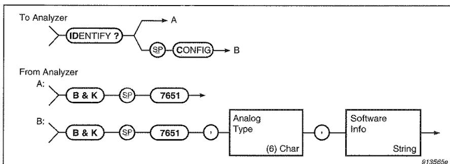
*Fig. 7.6 Syntax for the ID? query message and analyzer response*
