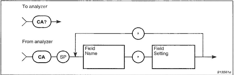
Fig. 6.8 Syntax for the CA? query message and analyzer response
