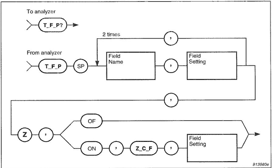
*Fig.6.6 Syntax for the T\_F\_P? query message and analyzer response*
