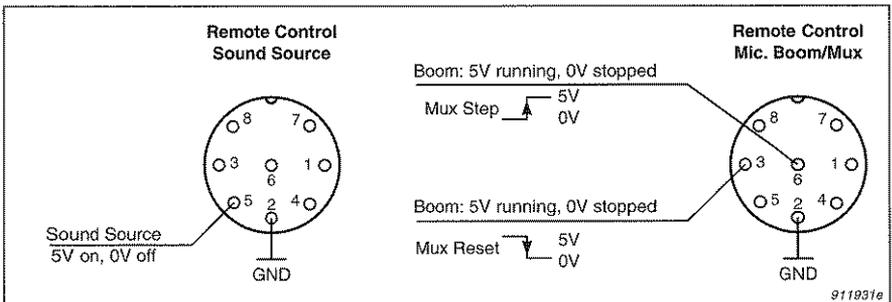
Fig. 3.4 Pin designations for Sound Source (left) and Microphone Boom/Multiplexer (right) connectors (outside view)
