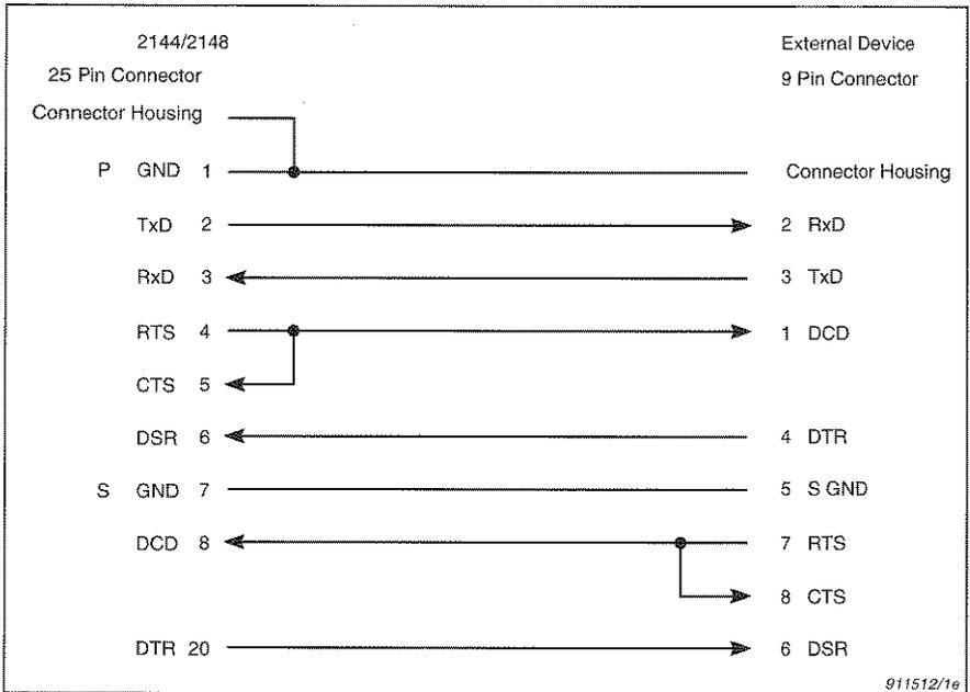
*Fig.3.4 Null-modem cable with one 25-pin connector and one 9-pin connector (Brüel&Kjær order number WL0945)*
