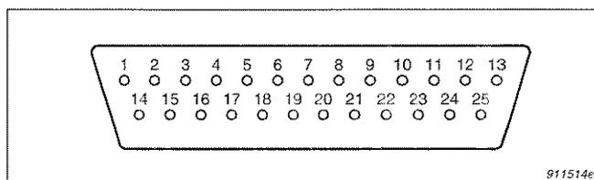
*Fig. 3.1 The RS-232-C interface connector of the 2148*
