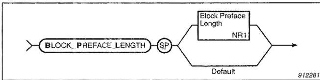
*Fig. 7.18 Syntax for the **B\_P\_L** command message*
