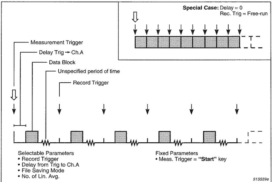
*Fig.5.5 Selectable parameters for data collection in Single Measurement mode*
