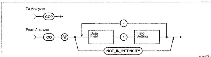
*Fig. 6.10 Syntax for the CO? query message and analyzer response*
