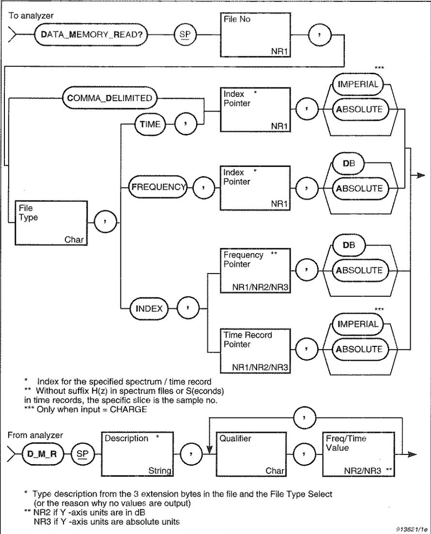
Fig.8.6 Syntax for the **D\_M\_R?** query message and analyzer response
