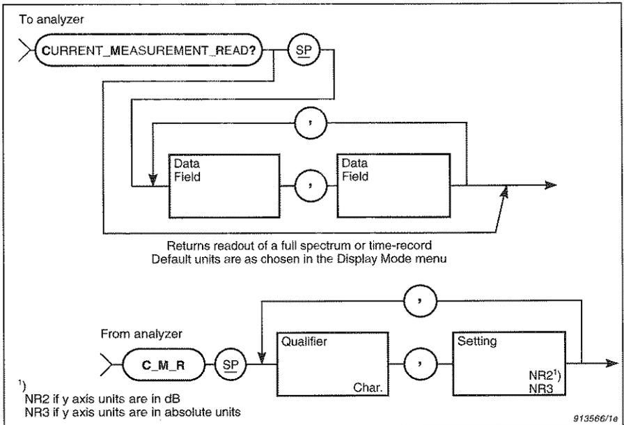
Fig.8.7 Syntax for the **C\_M\_R?** query message and analyzer response
