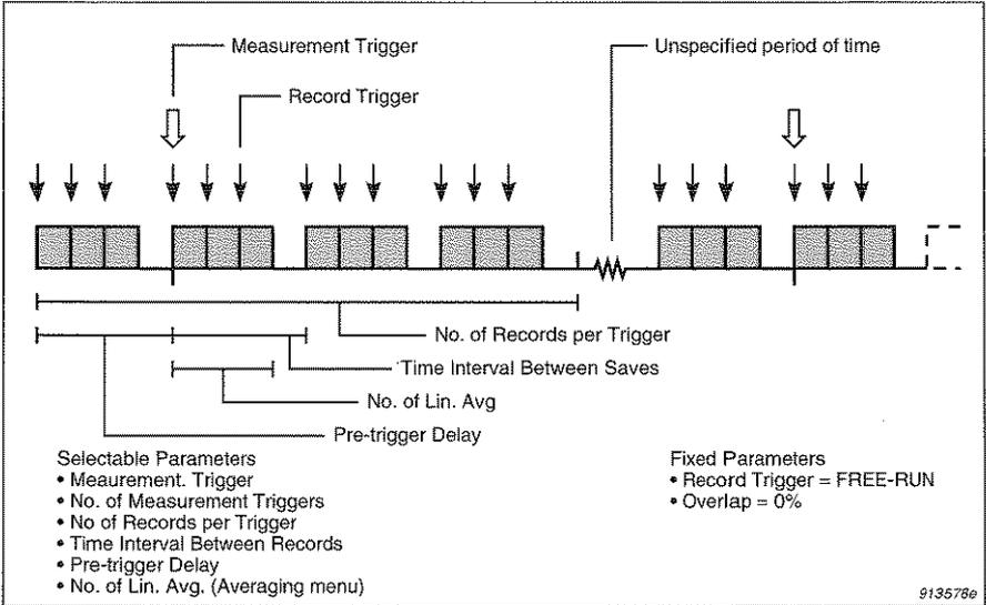
Fig.5.9 Selectable parameters for data collection in Time Capture mode (pre-trigger delay shown)
