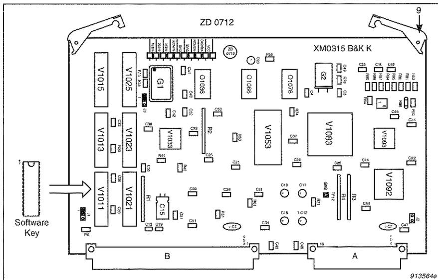
Fig.2.4 Position of software key on circuit board 9
