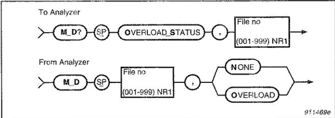
Fig. 6.34 Syntax for the **M\_D?** Overload query message and analyzer response
