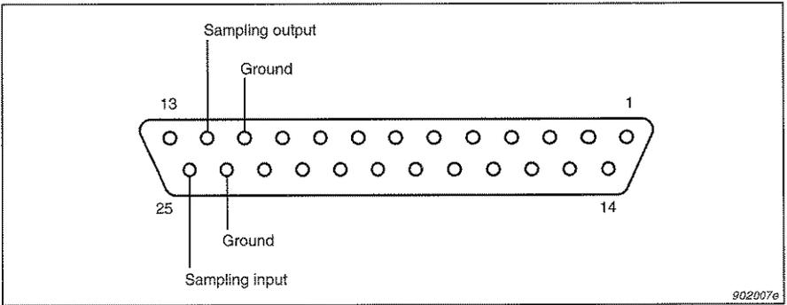
*Fig.3.3 Auxiliary Connector II (external view)*
