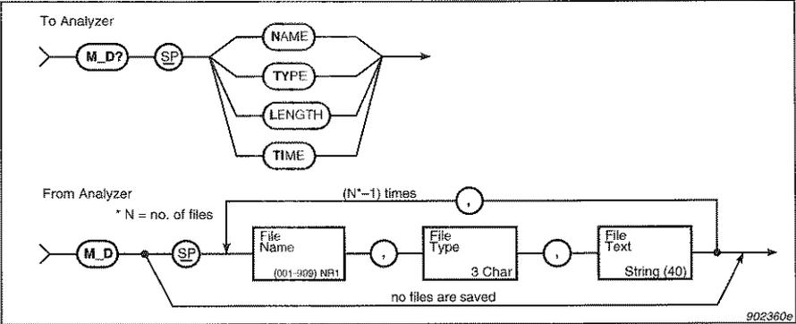
Fig. 6.33 Syntax for the **M\_D?** file list query message and analyzer response
