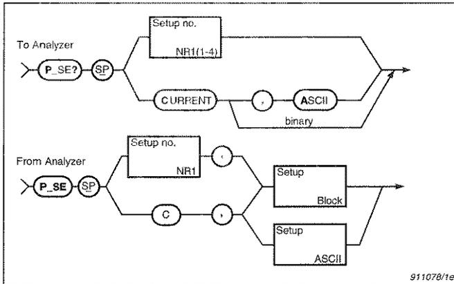
*Fig. 6.30 Syntax for the P\_SE? query message and analyzer response*
