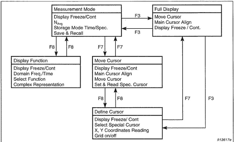
Fig.5.2 Measurement Mode menu structure showing the functions controlled from each menu
