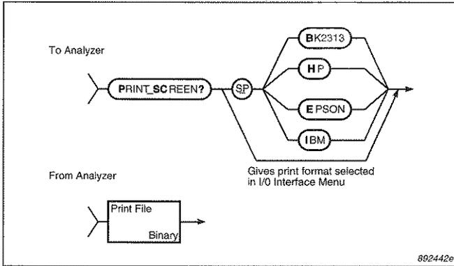
*Fig. 8.8 Syntax for the **P\_SC?** query message and analyzer response*
