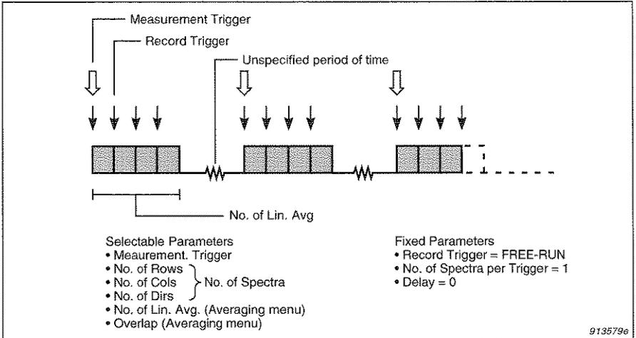
*Fig.5.13 Selectable parameters for data collection in Matrix Multispectrum mode*
