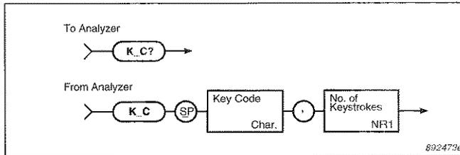
*Fig.5.3 Syntax for the **K\_C?** query message and analyzer response*
