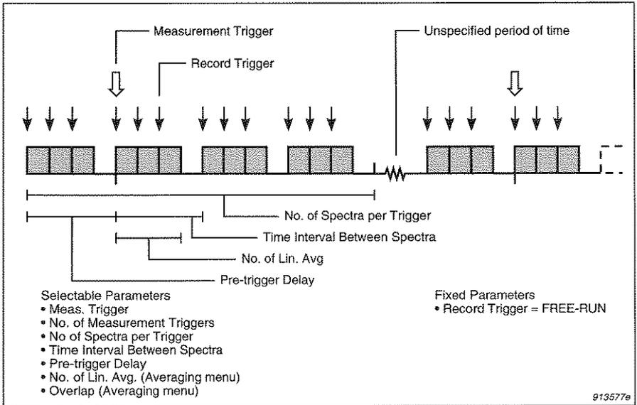
*Fig. 5.8 Selectable parameters for data collection in Normal Multispectrum mode (pre-trigger delay shown)*
