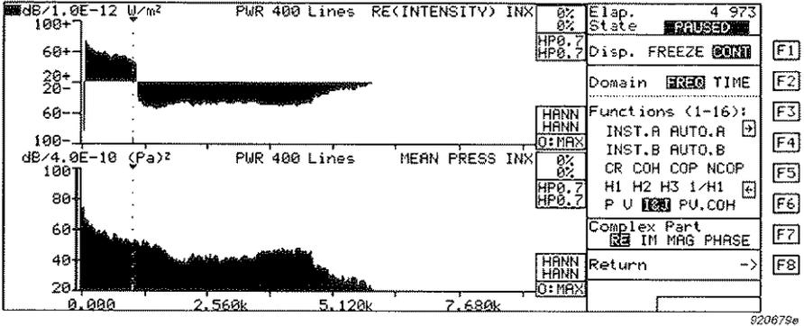
Fig.5.3 Display Function page for selecting which functions to display in Measurement Mode
