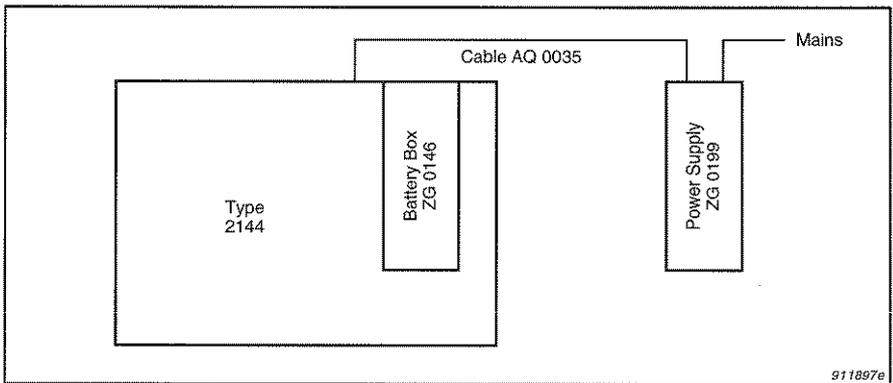
*Fig. 2.1 Arrangement for powering or recharging*
