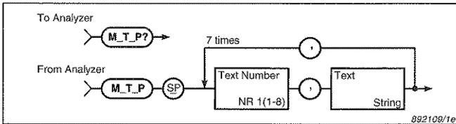
Fig. 6.24 Syntax for the M\_T\_P? query message and analyzer
