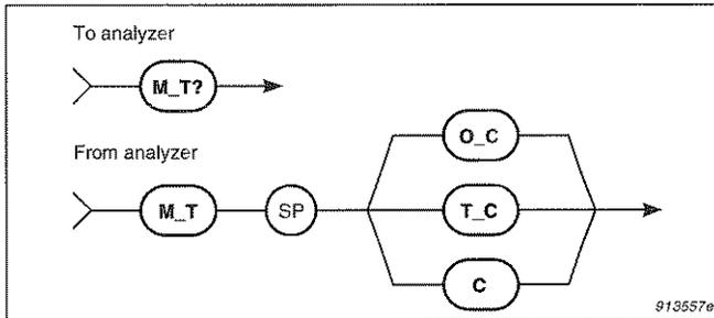
*Fig.6.2 Syntax for the **M\_T?** query message and analyzer response*
