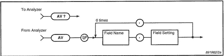
*Fig.6.12 Syntax for the AV? query message and analyzer response*
