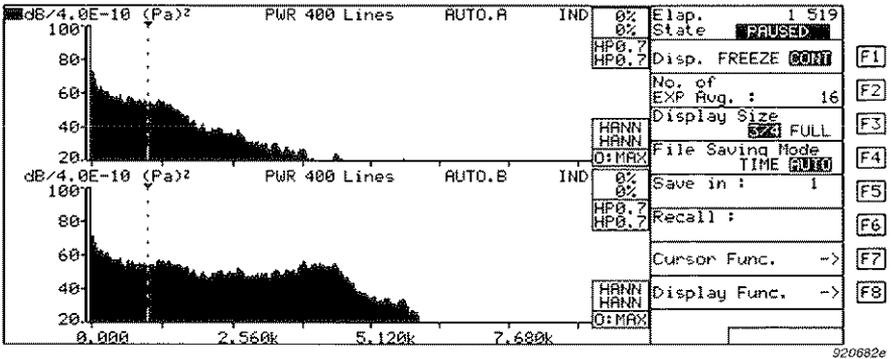
Fig. 5.1 A typical 2148 dual display in Measurement Mode
