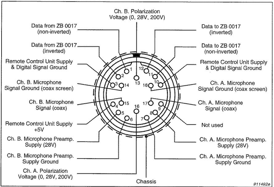
Fig.3.6 Pin designation for 18-pin Intensity Probe / Remote Control connector (outside view)
