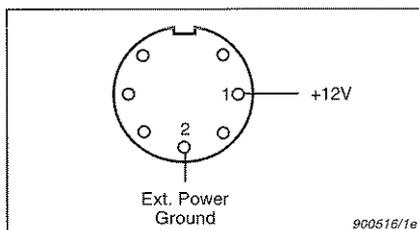
Fig. 3.8 Pin designation for 7-pin DIN external power connector (outside view)
