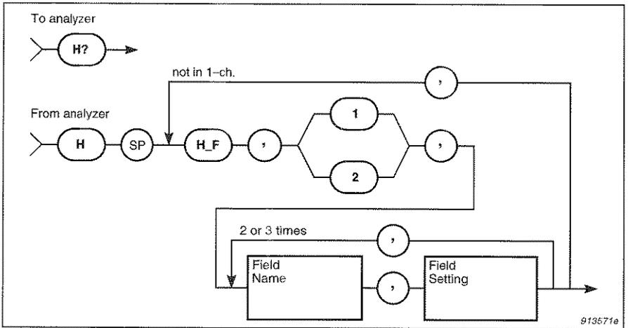
*Fig.6.16 Syntax for the **H?** query message and analyzer response*
