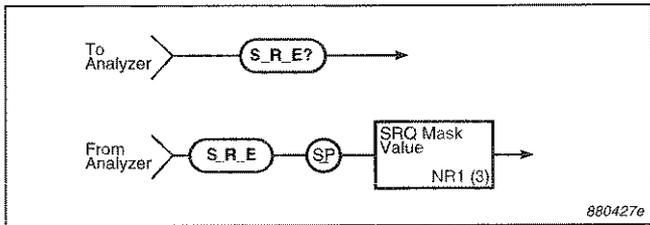
*Fig.7.2 Syntax for the S\_R\_E query message and analyzer response*
