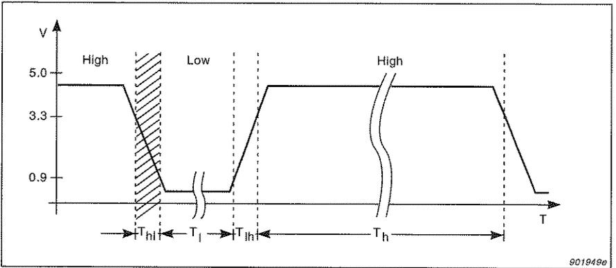
Fig.3.7 Trigger signal used for external triggering. Triggering occurs in the cross-hatched area
